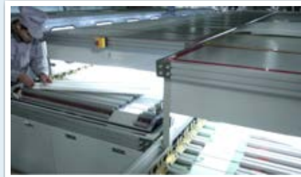
Aging Line for Tubes
